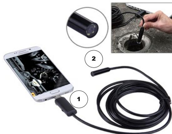
Figure 1 – Standard camera (1) mounts in the phone USB port, (2) 3 mm. camera with dimmable lights (image from Cellrizon)
